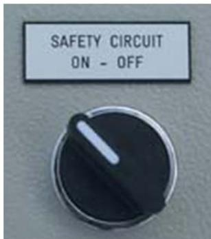
2. "SAFETY CIRCUIT" Schalter in Stellung "ON" schwenken.
