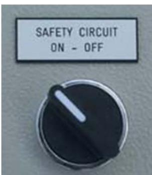
5. Den Schalter "SAFETY CIRCUIT" in Stellung "ON" schwenken.
